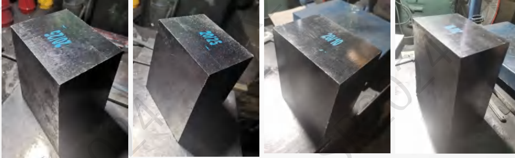
Fig. 5 sample magnesia-carbon brick prepared by Eco-friendly binder
